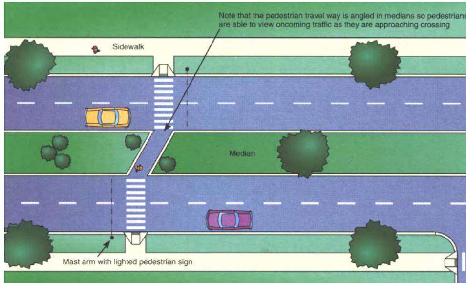
*A lowered median can be used to filter storm water and provide refuge for pedestrians crossing a roadway (Image from AASHTO).*
