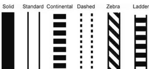
An engineering study may need to be performed to determine the appropriate width of a crosswalk at a given location, however marked crosswalks should not be less than six feet in width. In downtown areas or other locations of high pedestrian traffic, a width of ten feet or greater should be considered.
